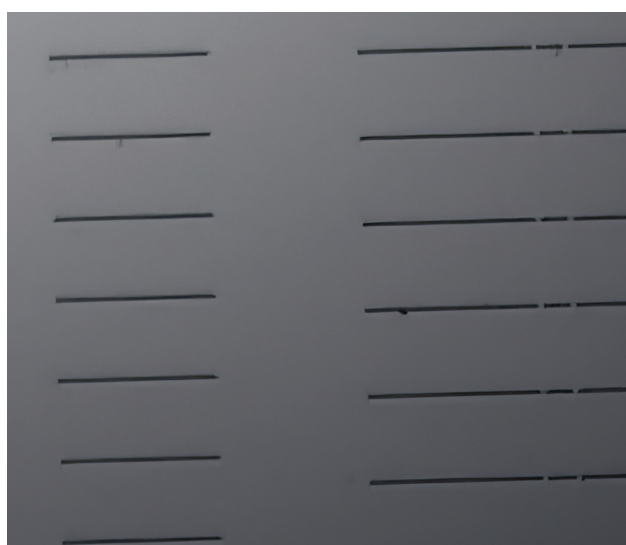
Fig. 1 A TRlton® system installed on an Oxford Instrument Plasma Technology chamber (upper image), and the camera captured an image (bottom) of an InP wafer's top surface, highlighting a test structure based on \sim 10 \mu\text{m} horizontal narrow strips spaced by \sim 400 \mu\text{m} .
