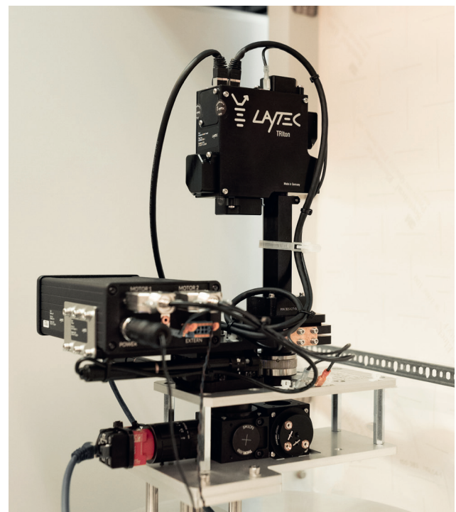
Fig. 1 LayTec's TRlton® in-situ metrology system for plasma etch monitoring installed on the top of an ICP chamber. In the lower part, TRlton's® optional camera for simplified measurement spot positioning can be seen.
