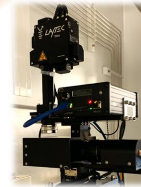
In-situ metrology during plasma etching
