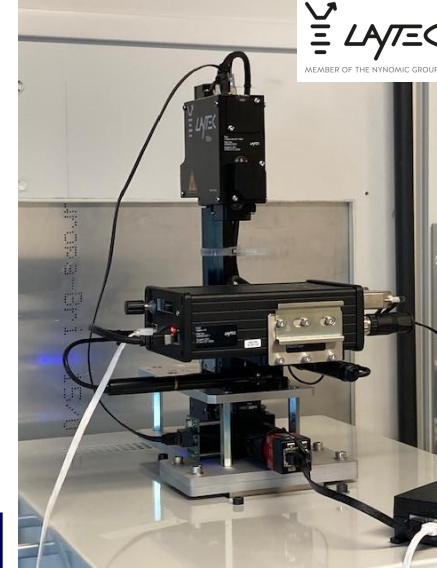
LayTec TRlton in-situ multi-wavelength metrology on top of the ICP etching tool
