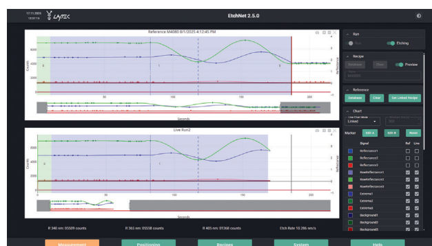
Figure 1: EtchNet measurement view showing the reference traces with recipe preview (top) and the live processing and predicted endpoint during an etch run (bottom).
