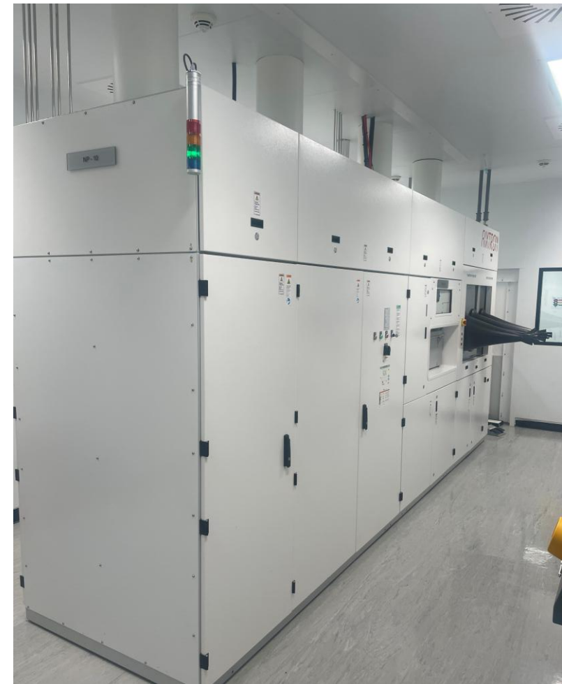
Aixtron G4 planetary reactor. IQE has 13 installed at its South Wales sites all with LayTec EpiTT systems
