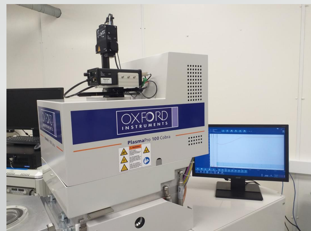
LayTec in-situ metrology applied for monitoring atomic layer etching processes
